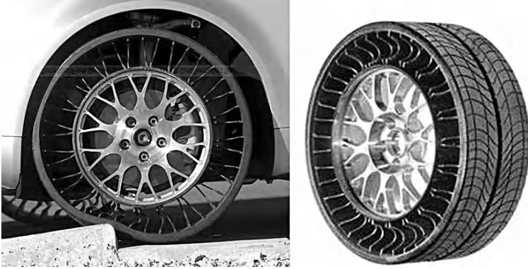
FIGURE 1.34. Twheel : an elastic non-pneumatic wheel recently developed by Michelin.
