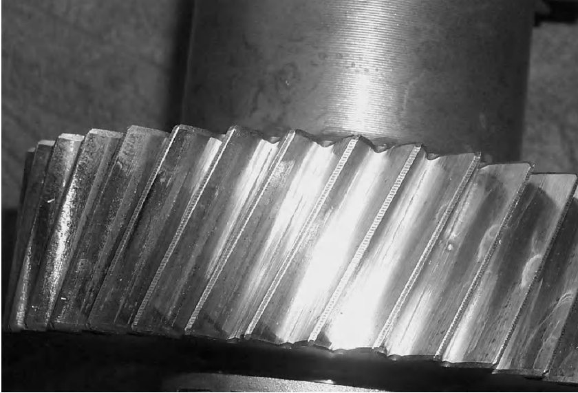
FIGURE 16.4. Aspect of a tooth flank damaged by pitting.
