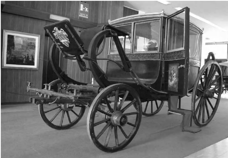
FIGURE 1.1. This coach built around 1650 shows the existence of a suspension; the sprung mass includes the passenger compartment only and is connected to the unsprung mass with four leaf springs with leader belts (Automobile Museum of Turin).
