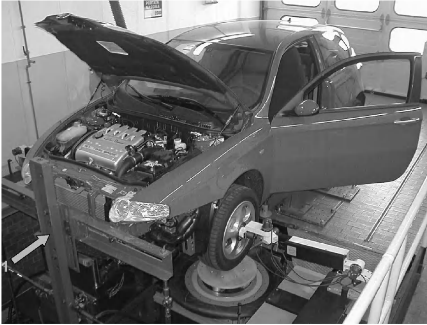
FIGURE 3.84. Elasto-kinematic bench with hydraulic actuators and anthropomorphic arm measuring system. The anthropomorphic arm detects the spatial wheel motion, consequent to force application or suspension stroke.
