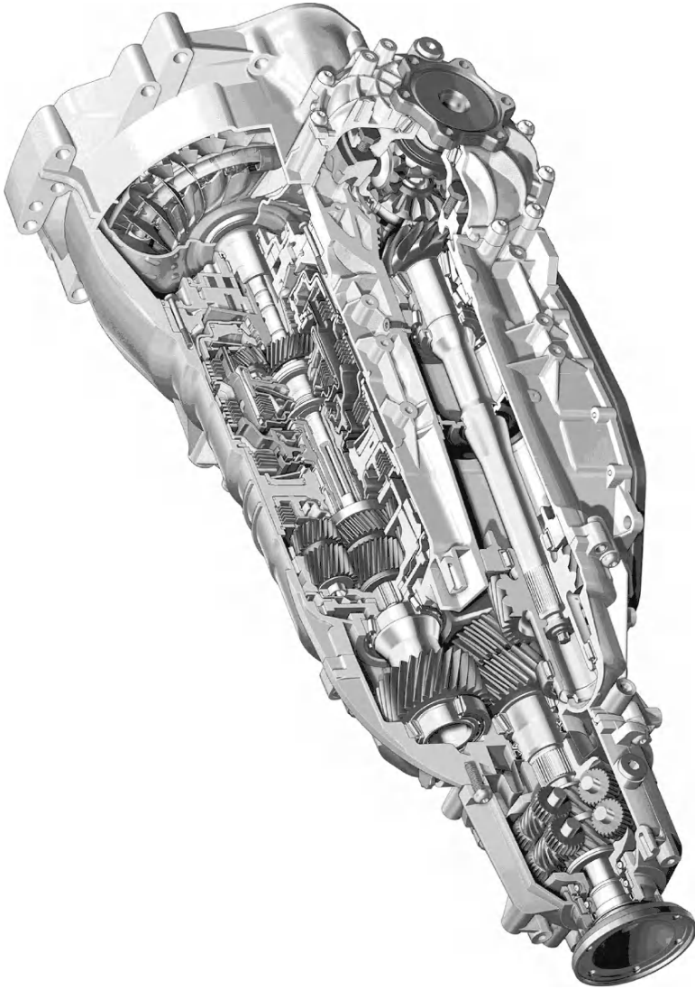
FIGURE 15.19. Six speed automatic gearbox with epicycloidal gear trains; the lateral shaft connects the gearbox output shaft with the differential pinion, behind the engine (Audi).
