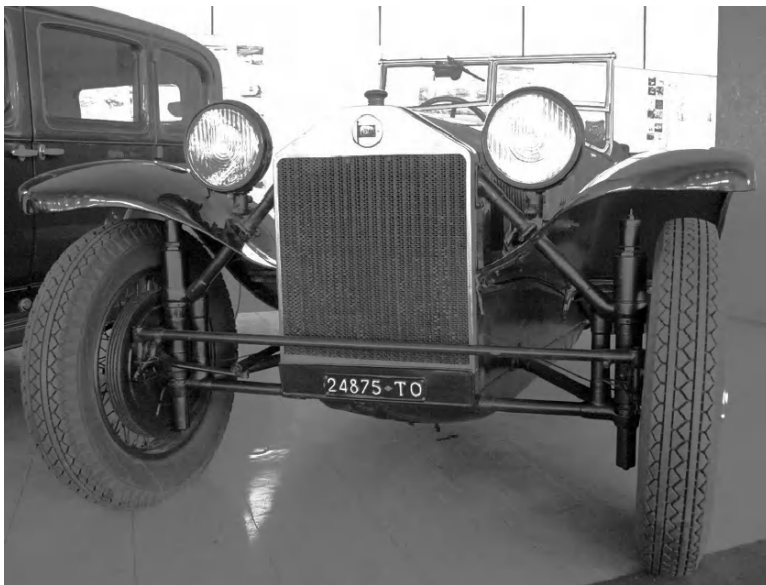
FIGURE 1.13. The front view of the Lancia Lambda shows the front suspension and the gate structure of connection to the body (Automobile Museum of Turin).
