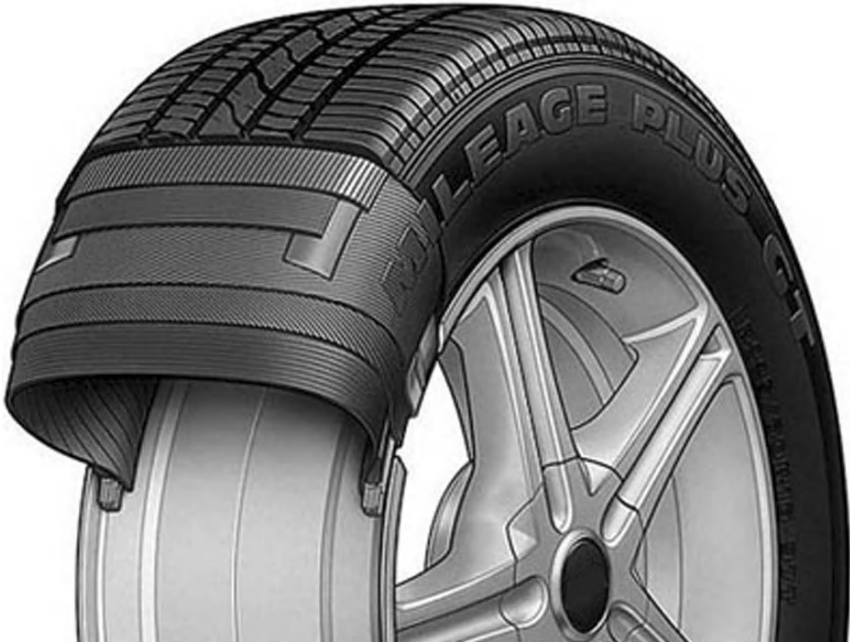
FIGURE 2.2. Radial tire structure: the tires include plies with circumferential cords (belt) and plies with radial cords (flanks) and two reinforcement cables in the bead for that part of the tire contacting the rim.
