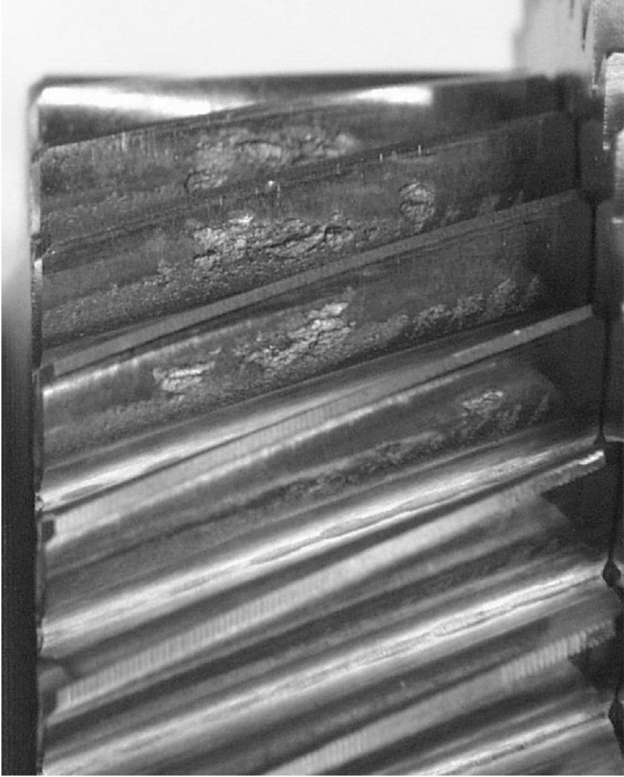
FIGURE 16.5. Aspect of a tooth flank damaged by heavy pitting.
