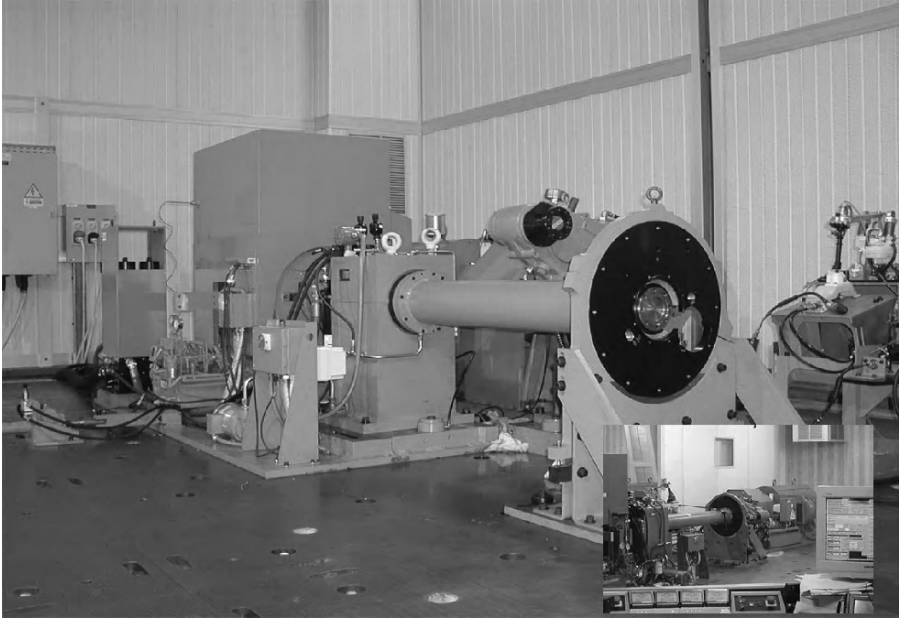
FIGURE 16.13. Interior of a typical modern test cell for complete transmissions. This kind of test cell can be adapted to all kind of tests, including acoustic emission measurement. It is acoustically reverberant, but can be changed to an anechoic cell, by encapsulating the transmission only in a suitable cabin.
