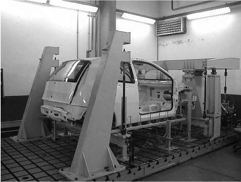
FIGURE 7.17. Universal bench prepared for torsion test; the articulated frame in the front is used to apply a roll torque.
