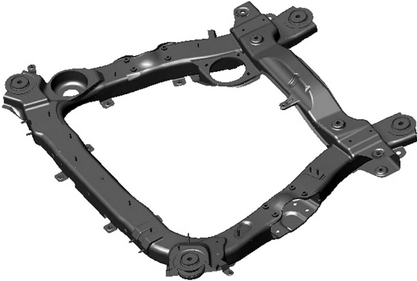
FIGURE 7.5. Perimetrical subframe for large front wheel driven cars; the front of the car should be imagined on the left side of the picture (Lancia).
