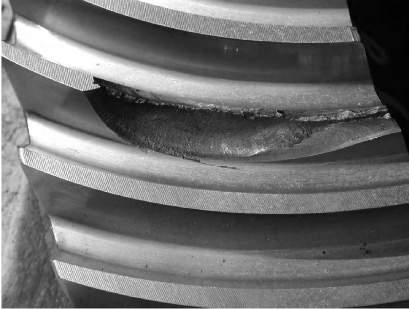
FIGURE 16.3. Appearance of a tooth flank damaged by bending fatigue.
